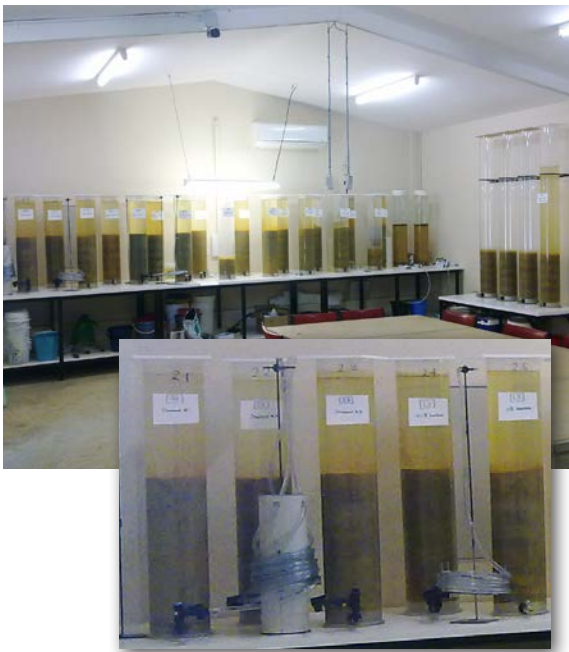
Figure 3 Column leach trials at the Brukunga Mine site used to test variables relating to the geochemical aspects of remediation. (Photo 409689)
