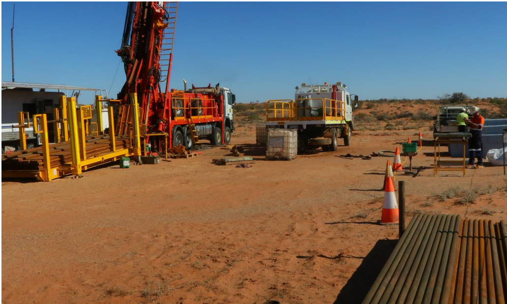
Figure 3. Example of drill site set up and equipment. The photograph of typical drill site showing (L to R) rod rack/sloop (on a hydraulic powered flatbed truck platform), driller office caravan, drill rig, support truck, core presentation and processing area.
