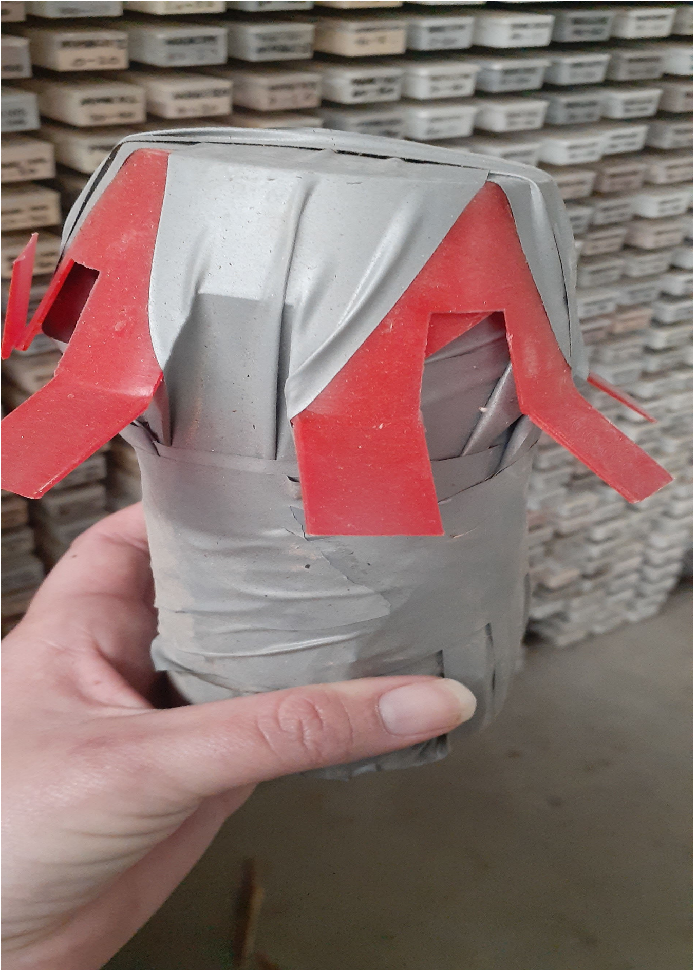
Figure 5. Custom made hole plug for cementing downhole
