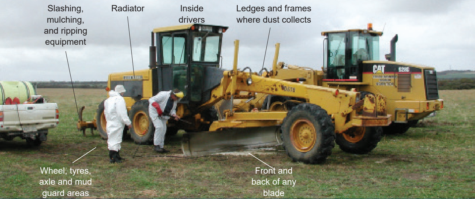
Decontaminate graders and ground engaging machinery
