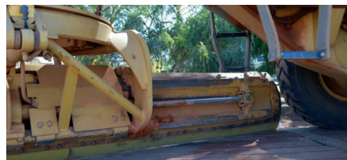
Decontaminate front and back of grader blades and hydraulic rods
