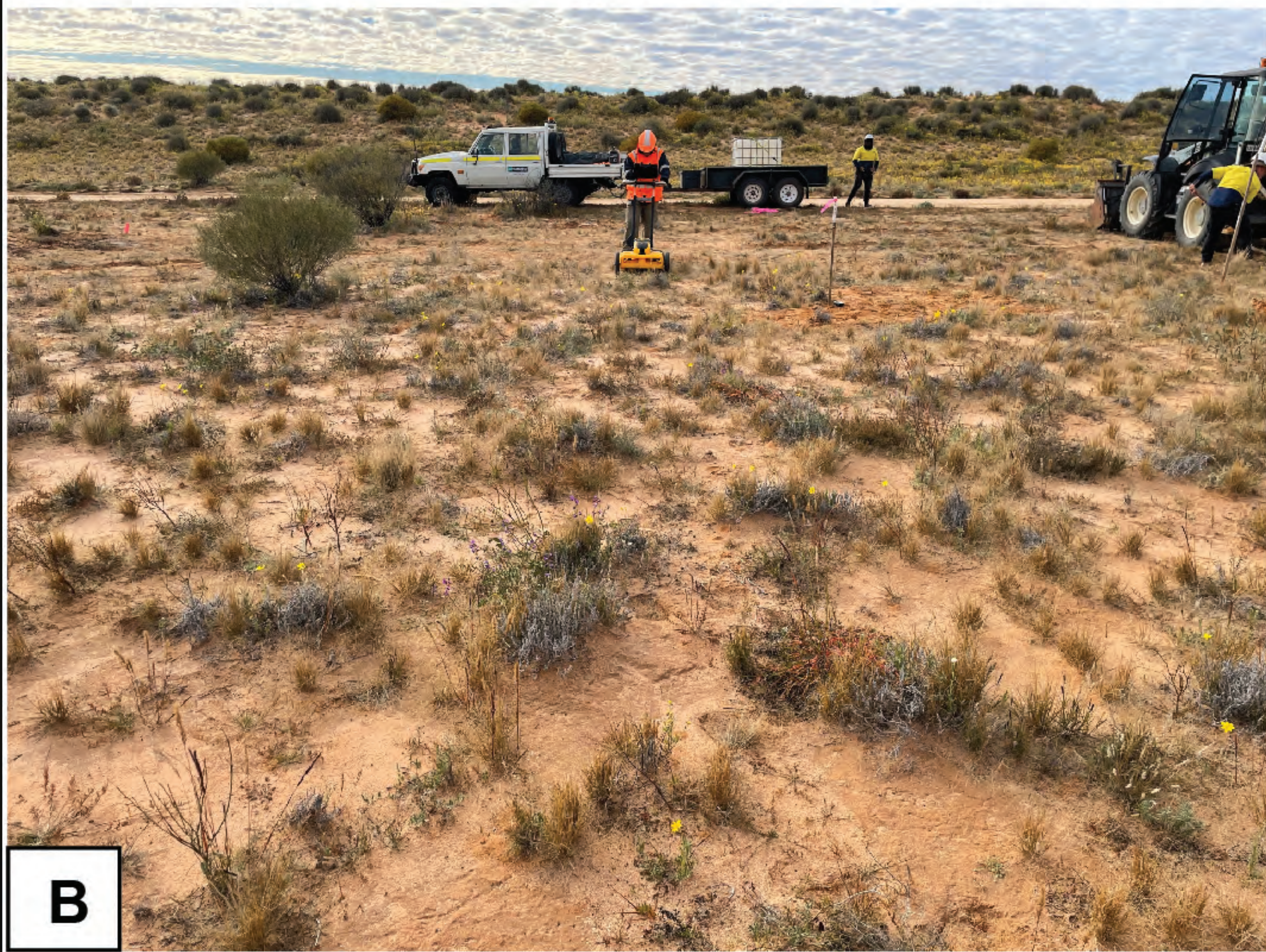
Above: Imaging the sub-surface using ground penetrating radar.
