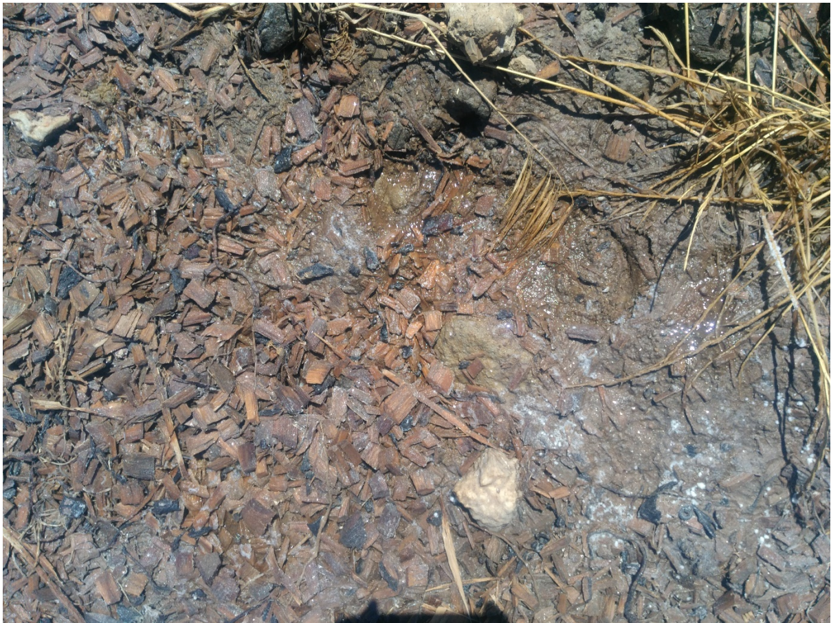
Photo 3: Seepage observed from the Transfer pond adjacent to pond PA11, 3 December 2020.
