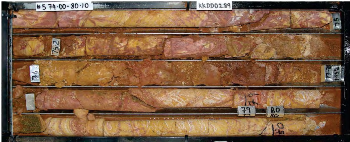
Figure 4-6 Core Photo of Weathered Saprolite Material (KKDD00289 74 to 80 m) (Kalkaroo Copper, 2021)
