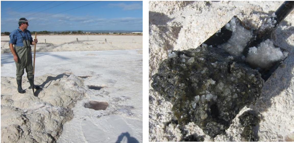
Figure 3 Photographs of pond PA12 showing salt crystals and crusts (gypsum and halite). This right hand picture also shows monosulfidic material present underneath the crusts.
