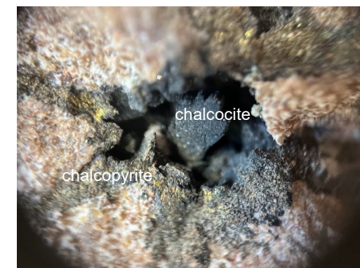
Infill sulphides in DH M350-250 @35m Pandurra Formation, Cattlegrid deposit
