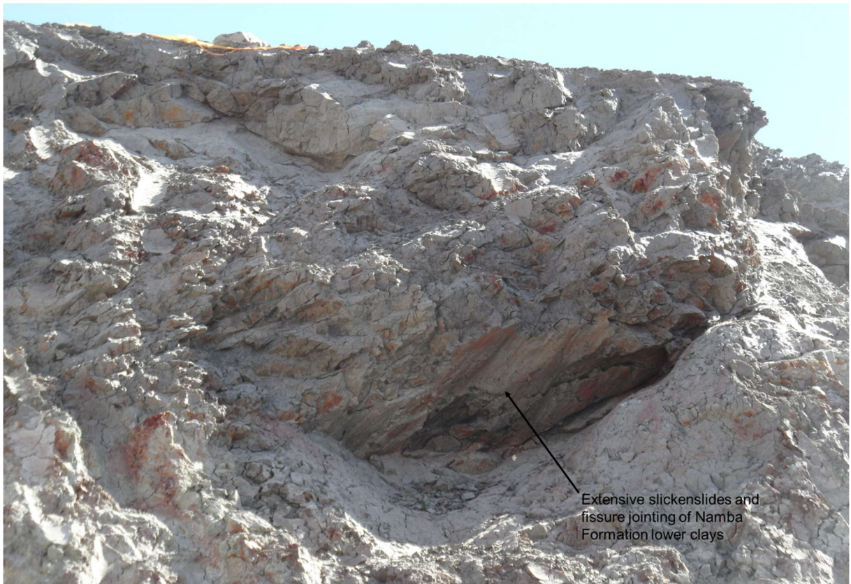
Figure 5. Recently exposed Namba Formation strata showing structure (fissuring and slickensides) of the smectite clay before drying.
