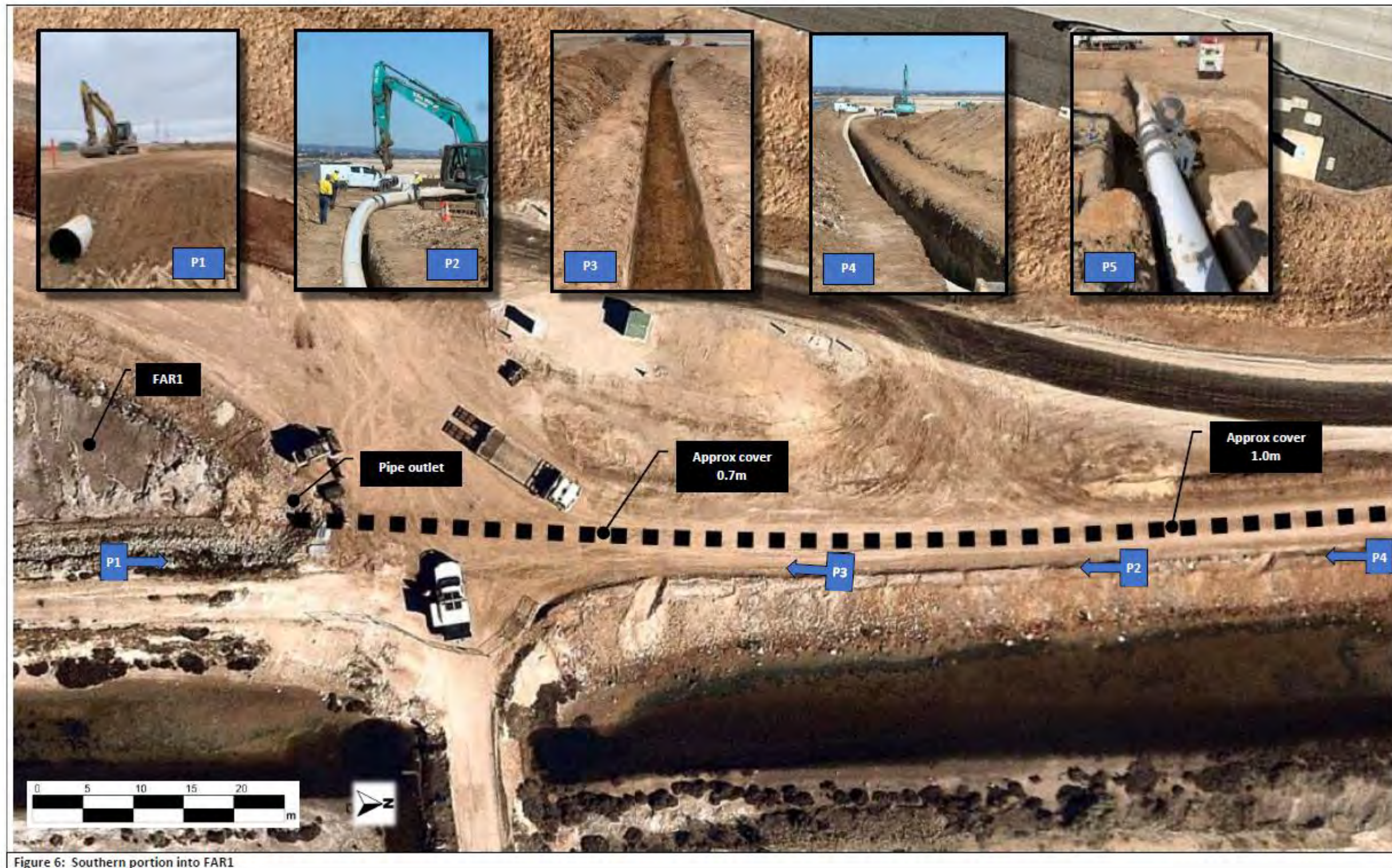
Figure 12-6: Information on Brine Pipeline from Section 2 to Section 1 – F
