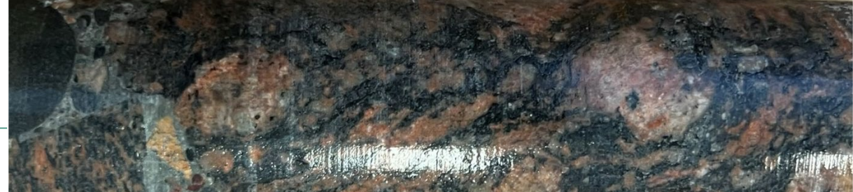
Permian diamictite core, Arckaringa Basin at 406-409 m with basement clasts
