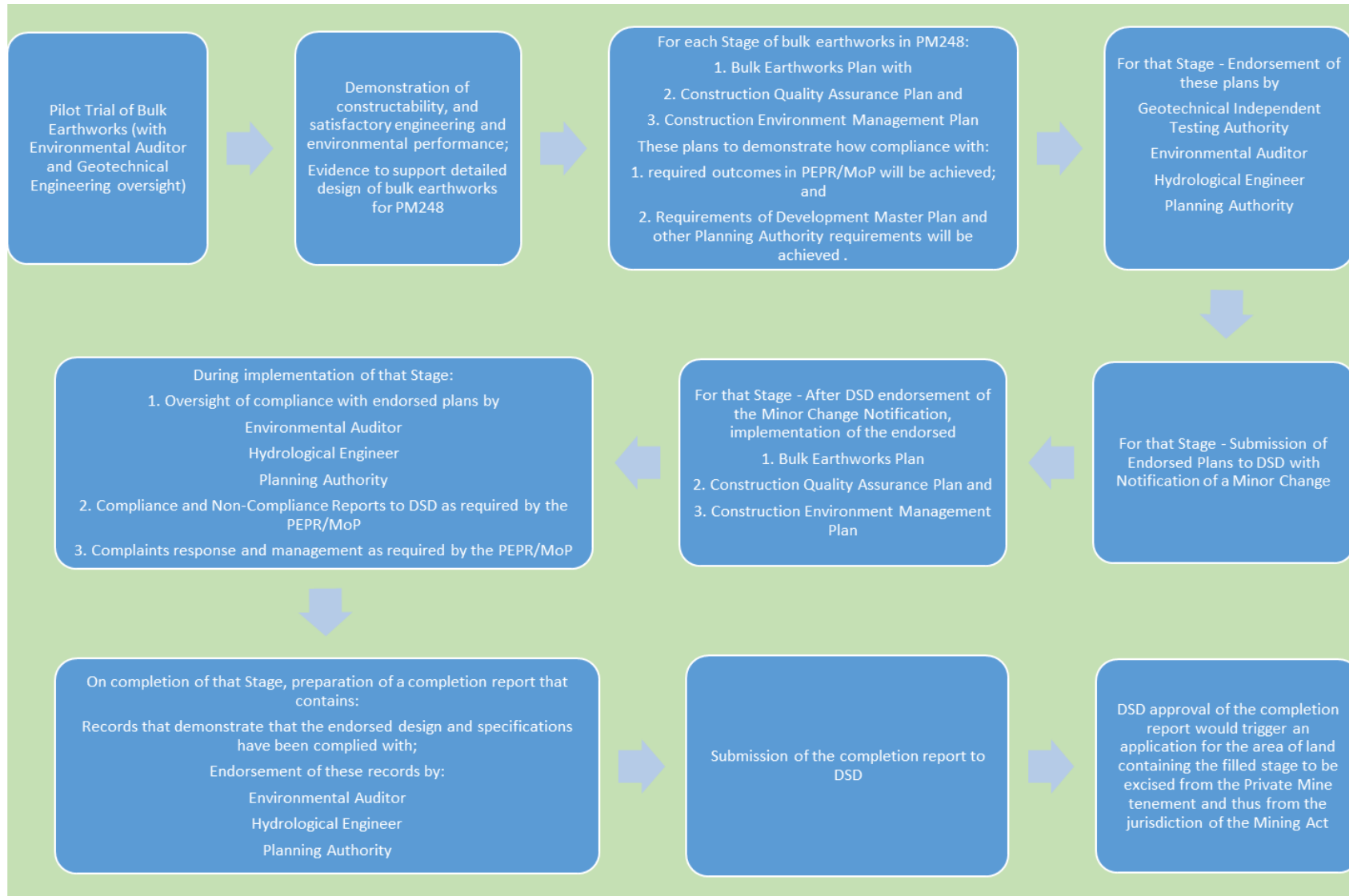
Figure 19-3: Process to manage and regulate bulk earthworks
