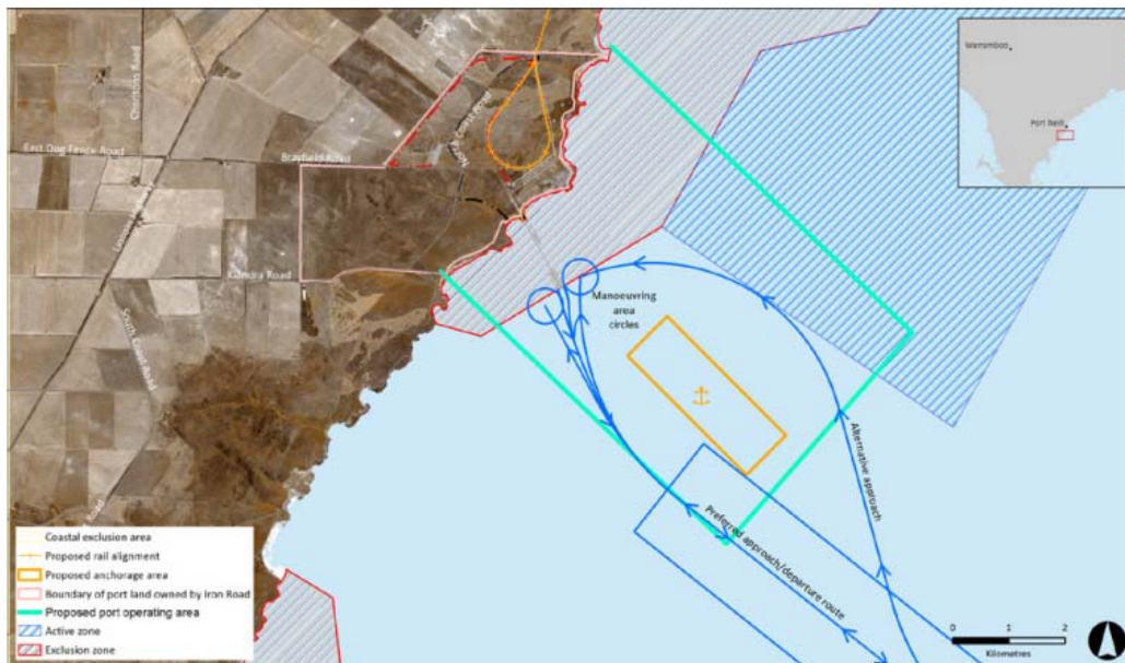
Figure 6 - port operating limits and anchorages - supplied image - 4.44 Iron Road EIS Chapter 4 page 4-69
