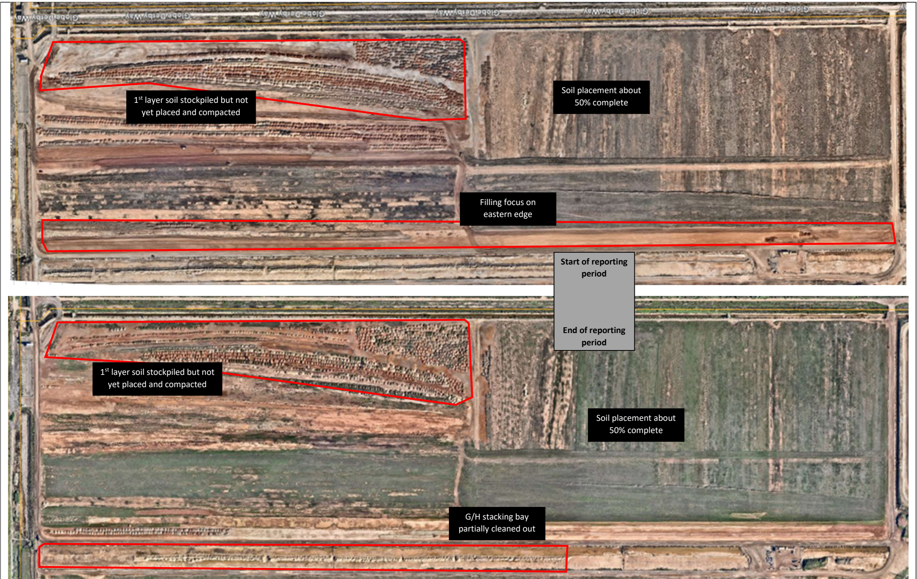
Figure 4: Filling status of G row at start and end of reporting period
