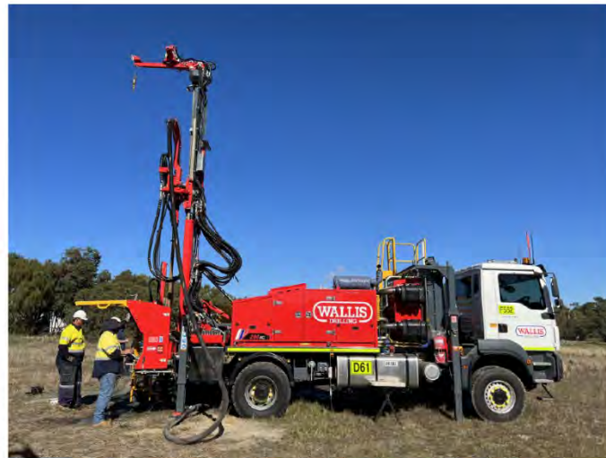
MANTIS 200 AIRCORE DRILL RIG
