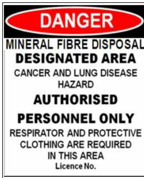
Figure 3: Signage to delineate areas of fibrous waste disposal.
