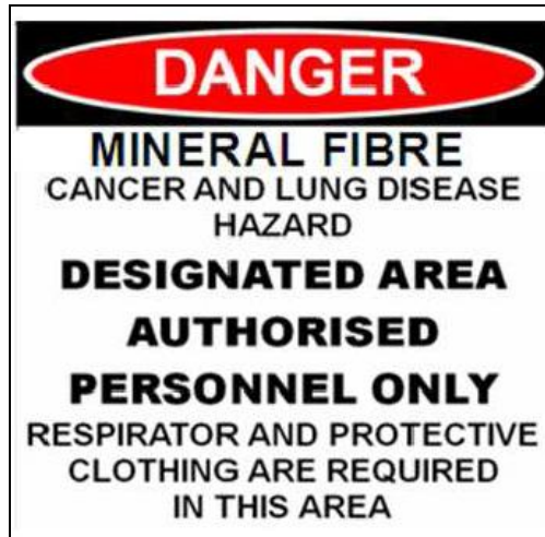
Figure 2: Signage to delineate active work areas in the presence of fibrous or potentially fibrous minerals.
