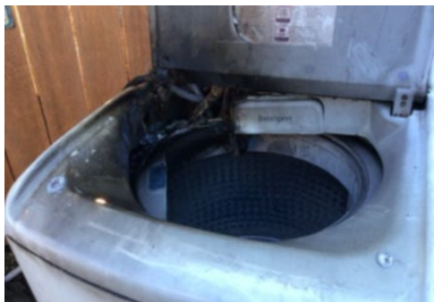
Figure E 10: Example of an electrical product failure
